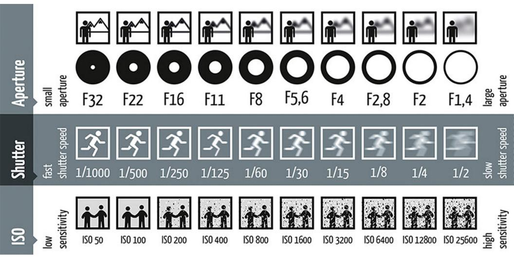
Aperture- how wide we open the hole in the back of the lens-measured in F Stops-A Small F-Stop # means a large opening- A Large F Stop # means a small opening
